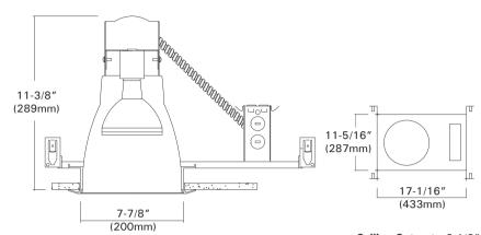
Ceiling Cut-out: 8-1/8" Lamp, Max, Watt.: 300W / R40, PS25 (Med, Mog) or 250W / PAR38 (Med) or 150W / A19 (Med)
